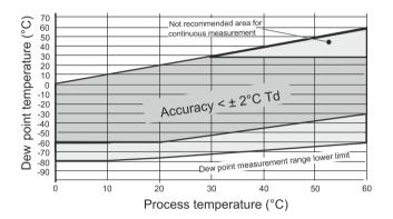
DEW POINT ACCURACY VS. MEASUREMENT CONDITIONS
